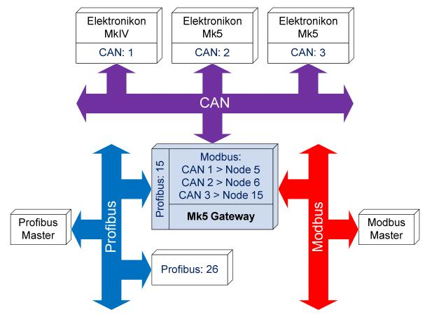
**NOTE**: the profibus manufacturer of the module must create a so named "Electronic Datasheet" or GSD file that declares the dimensions and the type of the exchanged datas. This file is public information necessary for Profibus users to interface with the bridge module.
