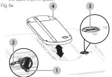
If the table insert is not level with the saw table, using a 2.5 mm hex key (not supplied), adjust the four set screws 5 pre-assembled to the table located on the four holes of the table insert until the table insert is level with the working table
