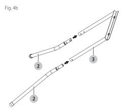
Lay outer leg assembly 1 2 on a flat surface. Place inner leg assembly 2 3 on top of outer leg assembly with the top rails facing each other. Angled ends of lower legs 2 should face away from each other so they resemble a "V".
