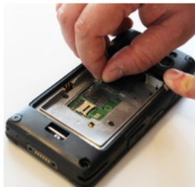
5. Insert the SIM card into the holder. Make sure the contacts side is face down:
