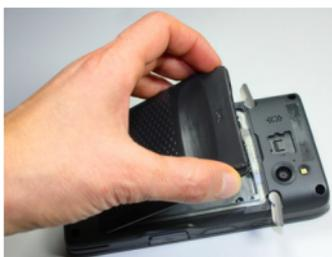
4. Remove the battery by pulling the tab on the bottom of the battery:
