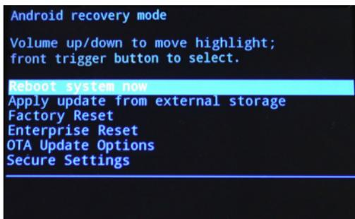
4. Use the volume buttons to navigate the menu. You can apply/force updates and perform a configuration reset. Press the front trigger to select.
