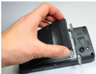
3. Remove the battery pack from the battery box\*. Insert the battery pack into the slot, top (contacts) side first, and press it into place:
