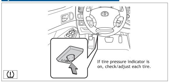
After adjusting tire pressures, or after tires have been rotated or replaced, turn the ignition switch to "ON" and press and hold the " SET" button until indicator blinks three times. Let the vehicle sit for a few minutes to allow initialization to complete.
