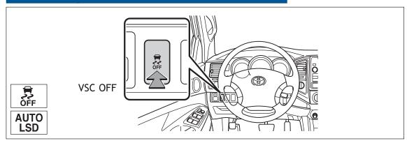
The VSC OFF switch is used to switch between modes related to the TRAC, VSC and Auto LSD functions.
