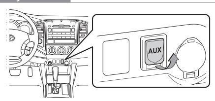
Push "DISC. AUX" button after inserting a mini plug into the AUX audio jack to listen to music from a portable audio device through the vehicle's speaker system while in AUX mode.
