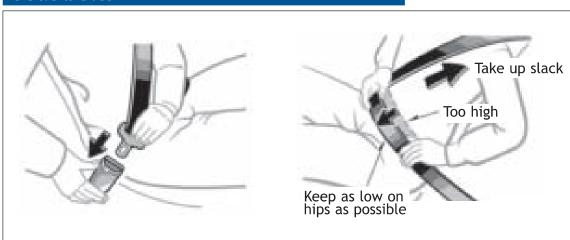
If belt is fully extended, then retracted even slightly, it cannot be re-extended beyond that point, unless fully retracted again. This feature is used to help hold child restraint systems securely.
