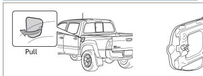
NOTE: Tighten until one click is heard. If the cap is not tightened enough, Check Engine " check " indicator may illuminate.
