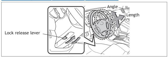
Hold wheel, push lever down, set angle and length, and return lever.
